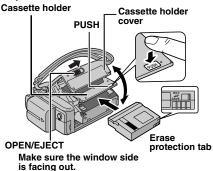
1 Slide and hold **OPEN/EJECT** in the direction of the arrow, then pull the cassette holder cover open until it locks. The cassette holder opens automatically.
